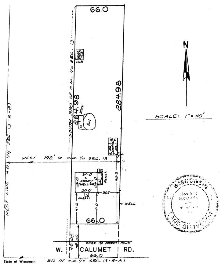
I have surveyed the above-described property and the above map is a true representation thereof and shows the size and location of the property, its exterior boundaries, the location and dimensions of all structures thereon, fences, apparent easements and roadways and visible encroachments, if any
